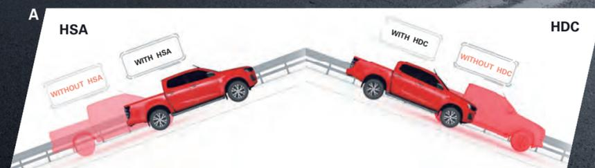
[A] **HSA and HDC:** Hill Start Assist and Hill Descent Control ensure maximum confidence in uneven terrain.
